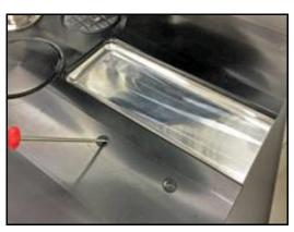
Spear and remove the two screw caps (Part no. 103628) which cover the threads of the print head fixing points using a thin screwdriver.
