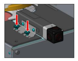
Fix the printhead onto the MEDIAJET using the two knurled head screws (2).
