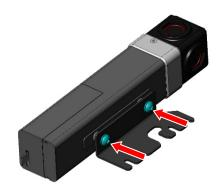
Fix the Mounting bracket (1) to the MI 9232/9410 inkjet printhead using the two M6x10 lens head screws (3) and the two Washers (4).
