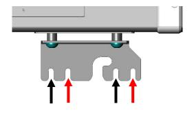
Use the anterior slots (black arrows) when printing on 90 mm Petri dishes or use the posterior slots (red arrows) when printing on 60 mm Petri dishes to fix the Mounting bracket (1) onto the MEDIAJET.
