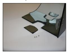
Remove the slot cover on the back side of the MEDIAJET Plexiglas safety cover.
