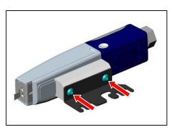
Fix the Mounting bracket (2) to the Printer head retainer (1) connected to the Domino inkjet printer head using the two M6x10 lens head screws (4).
