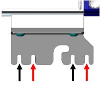
Use the anterior slots (black arrows) when printing on 90 mm Petri dishes or use the posterior slots (red arrows) when printing on 60 mm Petri dishes to fix the Mounting bracket (1) onto the MEDIAJET.
