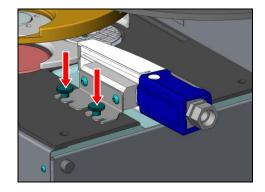
Fix the printer head onto the MEDIAJET using the two knurled head screws (3).
