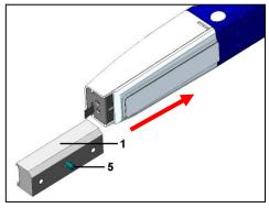
Slide-in Printer head retainer (1) onto Domino printer head and fix it using the Setscrew M5x16 (5).
