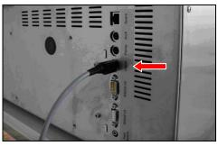
Insert the Mini-DIN 8 poles plug of the Interface cable (103082) into the socket labeled with INKJET on the rear panel of the MEDIAJET.
