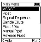
Select the ASSIST mode in the Main Menu of the VIAFLO pipette and press **OK**. The pipette establishes the Bluetooth connection.
