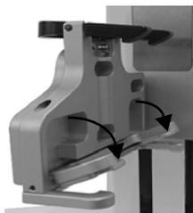
To adapt the holder for an 8- or 16-channel pipette, pull the silver lever down as shown beside.
