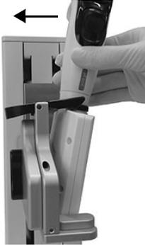
To install a pipette, hold it at an angle and insert it into the pipette holder.
