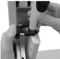
To release the VIAFLO Electronic Pipette lift the black gripper by pushing down on one end.
