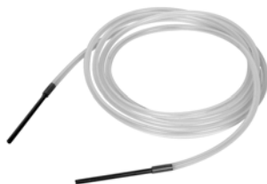
Silicone tubing set, consisting of silicone tubing 3.0 mm ID, 2.5 m length, stainless steel aspirating and dispensing tube, each of 10 cm length.
