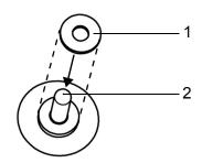
▶ Insert the disk (1) into the cuvette by putting it onto the pivot pin (2). Push it fully downwards to the bottom.
