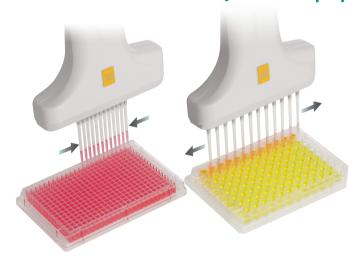
The VOYAGER II is the only pipette where the tip spacing can be changed electronically.
