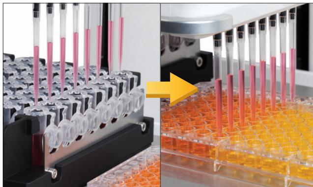
Equipping the ASSIST PLUS with a VOYAGER pipette enables on-the-fly adjustment of tip spacing, allowing multichannel sample reformatting – eg. from tubes to plates – and access to various labware types.
