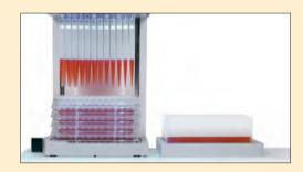
The "Repeat Dispense" mode allows for a very efficient filling of multiple microplates with the same liquid.
