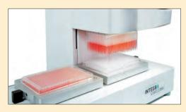
An exact aspiration height can be defined to precisely remove supernatant and ensures pipette tips do not impact the bottom of a plate.
