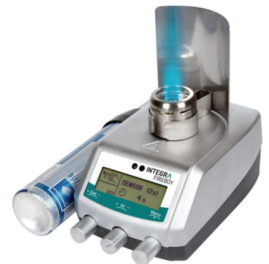
Typical safety Bunsen burner operated with a gas cartridge. This burner offers users the choice to ignite the flame by an infrared optical sensor, a foot switch or a push button on the instrument.
