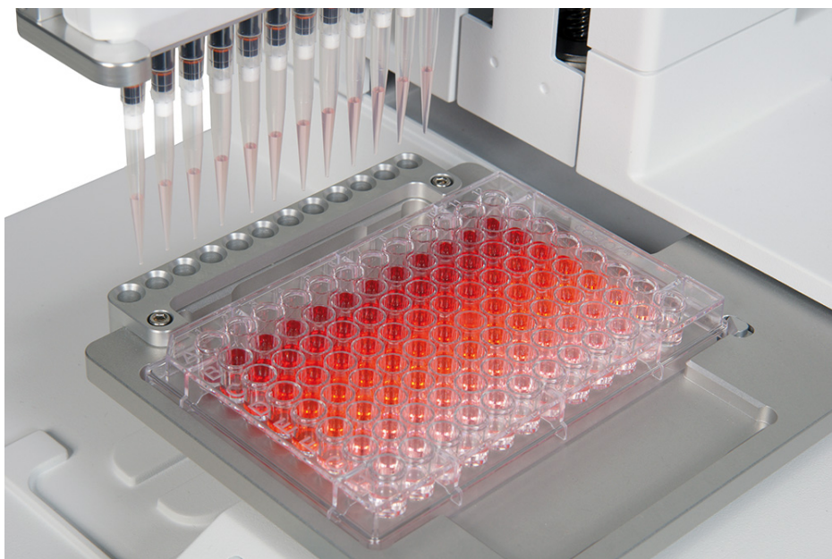
Caption: VIAFLO ASSIST automating serial dilution on a 96-well plate
