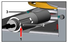
**LINX CJ400/89xx**, printhead **MK11:** Insert the printhead into the Printhead retainer and align the screw (1) of the printhead with the <u>forefront</u> notch (2) of the retainer. Fix the printhead with the Allen screw M4x8 (3).
