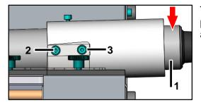
Tighten the anterior Allen screw M4x8 (2). Push the printhead (1) to the <u>lower stop</u> of the posterior screw hole and tighten the Allen screw M4x8 (3).
