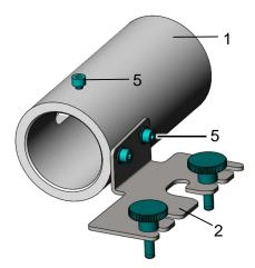
Screw one Allen screw M4x8 (5) on the Printhead retainer (1) and mount the Mounting bracket (2) on the Printhead retainer (1) with two Allen screws M4x8 (5).
