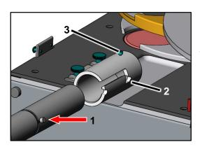
**LINX 4900/5900**, printhead **MK7:** Insert the printhead into the Printhead retainer and align the screw (1) of the printhead with the <u>furthest</u> notch (2) of the retainer. Fix the printhead with the Allen screw M4x8 (3).
