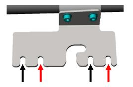
Use the anterior slots (black arrows) when printing on 90 mm Petri dishes or use the posterior slots (red arrows) when printing on 60 mm Petri dishes to fix the Mounting bracket (2) onto the MEDIAJET.
