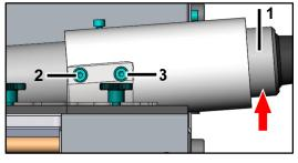
Tighten the anterior Allen screw M4x8 (2). Push the printhead (1) to the <u>upper stop</u> of the posterior screw hole and tighten the Allen screw M4x8 (3).
