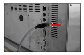
Insert the Mini-DIN 8 pole plug of the Interface cable (Part no. 113853) into the socket labeled with INKJET on the rear panel of the MEDIAJET.
