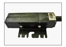
Fix the printhead adapter to the MI inkjet printhead using the two M6x10 Allen screws.
