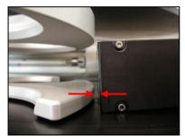
Mount the rotor to the MEDIAJET and check whether the clearance between the rotor and the printhead is between 1.5 to 3.5 mm.
