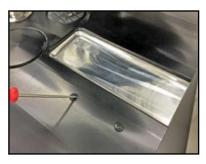
With a thin screwdriver spear the two round plastic pieces which cover the threads of the printhead fixing points and remove them.
