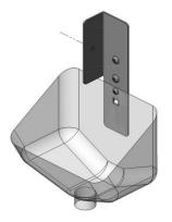
If you have a Maintenance tray to rinse the printhead, mount Printhead holder (103483) with Lens head screw M5x10, as shown beside.
