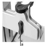
Set the lever (a) to the center to pipette in 96 well plates.
