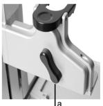
The front position of the lever (a) moves the pipette to the front to accommodate the front positions of 384 well plates.
