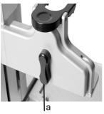
Set the lever (a) to the center to pipette in 96 well plates.
