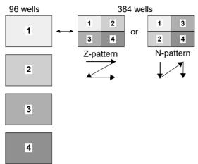
Reformat four 96 well source plates with an 8 channel VOYAGER pipette into 4 quadrants of one target 384 well plate.
