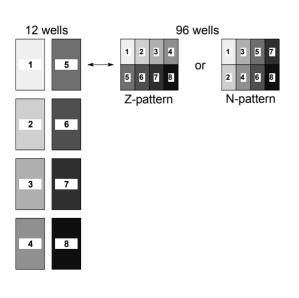
Reformat eight 12 well source plates with a 4 channel VOYAGER (300 µl) into 8 quadrants of one target 96 well plate.
