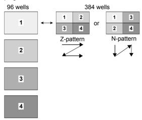
Reformat four 96 well source plates with an 8 channel VOYAGER pipette into 4 quadrants of one target 384 well plate.
