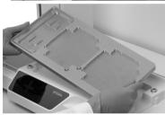
Hold the **Deck** (7) with both hands and place it over the corresponding positioning studs. Press down firmly until you hear a click.
