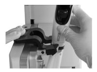
To release the pipette lift the black gripper by pushing down the left end.
