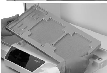
Hold the **deck** (7) with both hands and place it over the corresponding positioning studs. Press down firmly until you hear a click.
