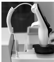
Click in the 4-pin of the communication cable to the pipette back and plug in the cable to the pipette holder of ASSIST PLUS.
