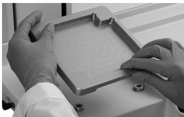
Hold the front and the back of the **tip rack deck** (6), find the correct orientation and place it over the corresponding positioning studs. Press down firmly until you hear a click.
