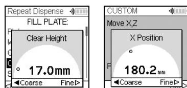
If the exact values of heights or X/Y/Z positions are known, they can be entered directly using the Touch Wheel.
