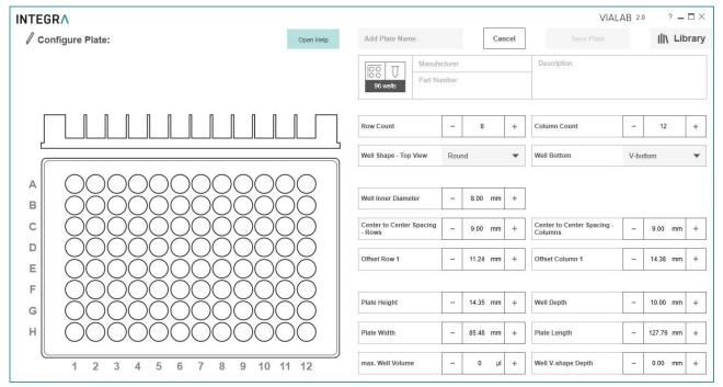
**Note:** For plates in adapters, e. g. in PCR 96 or 384 well cooling plates, define the dimensions of the inserted plate in combination with the adapter as one plate.
