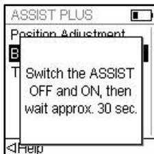
The first time a specific pipette is connected to ASSIST PLUS, both instruments need to be paired.
