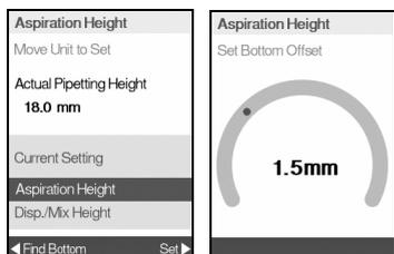
Select ◀ Find Bottom. Confirm that GRIPTIPS are attached. Set the bottom offset and confirm with **OK**.
