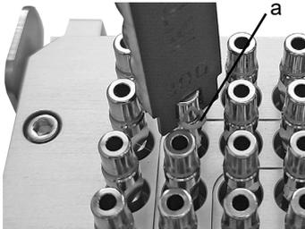
Place the O-ring removal tool vertically between the tip fittings (do not tilt).
