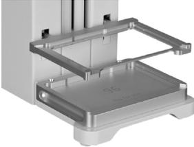
To install the **second stage**, remove the two **magnetic covers** (3) by pressing on one side or using a GRIPTIP. Insert the **second stage** with the desired side (96 or 384 format) facing upwards.
