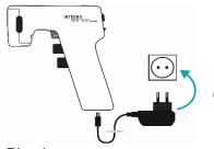
Charge the LiPo battery completely before first use.
