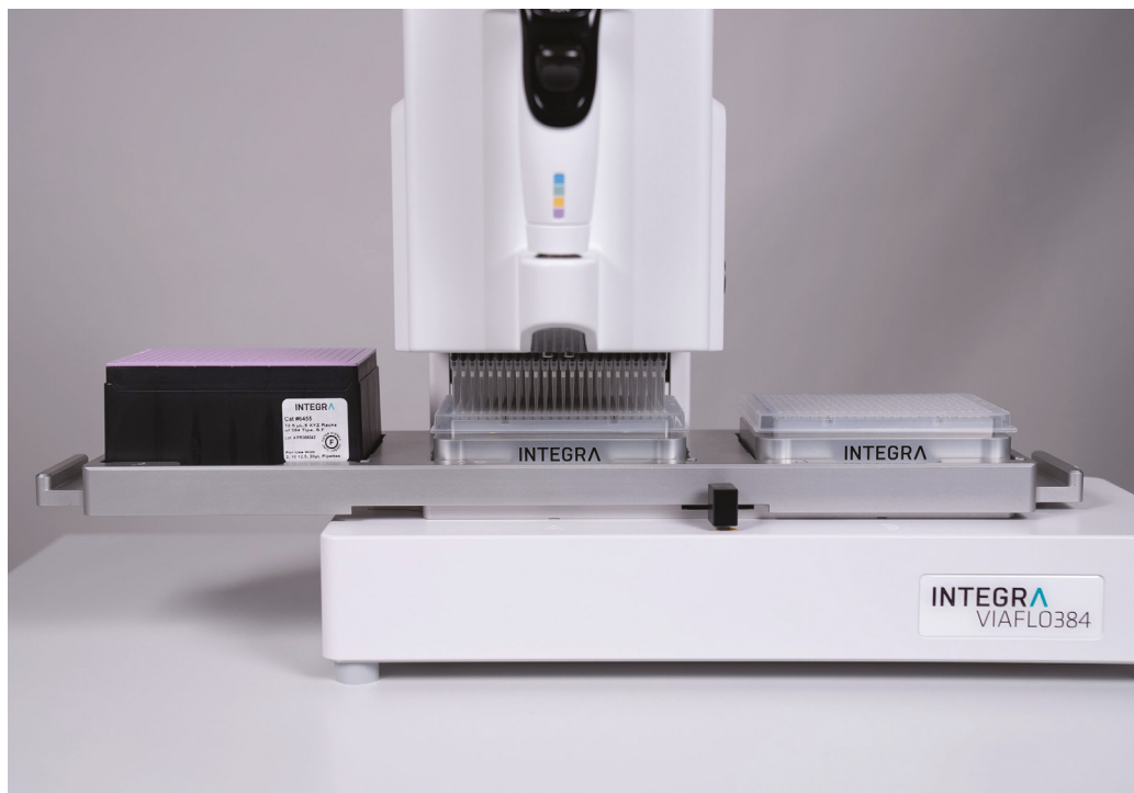
Figure 4: The three position stage of the VIAFLO 384 set-up for the barcoding step.
