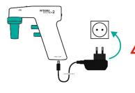
Charge the Li-ion battery completely before first use.
