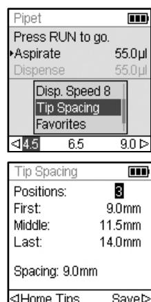
In each pipetting mode, the available tip spacing positions are displayed at the bottom of the screen. The current position is highlighted.
