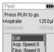
Insert the GripTips into the liquid to be transferred. Press and release the Run Key to aspirate the volume selected in the first step (marked with a triangle on the Run screen).
