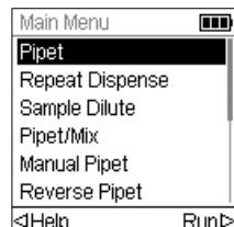
From the Main Menu, use the Touch Wheel to scroll to your desired function-based programming mode. Press OK to enter the mode and to start defining parameters.
