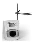
Fix the retort rod with the two screws on the rear side, using a Phillips screwdriver (PH2), see "Screw threads for fixation of the retort rod" on page 10.
