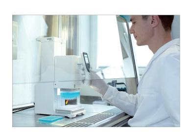
INTEGRA'S MINI 96 is the most affordable and portable 96 channel pipette – making your pipetting much faster and more reproducible vs. a traditional 1-16 channel pipette.
