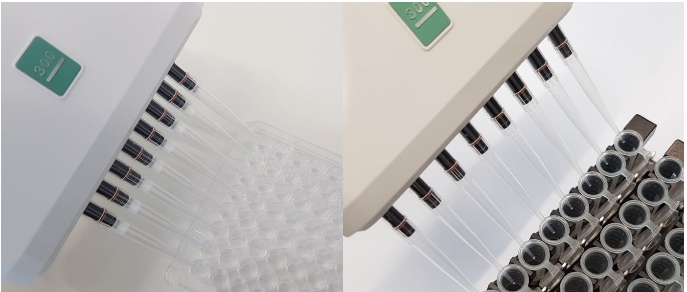
Figure 1: Adjust the tip spacing by aligning it against the empty 96 well plate and tube rack.
