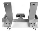
From the back of the stacker put the support brackets on the top of the Stacker Base and pull them to their stop.
