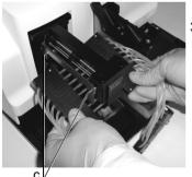
3) Hold the black left and the right dispensing cartridge below the rollers of the pump head, so that the tubings points downwards and the screws upwards. Fit the two holes on the inside of the left cartridge (<u>28</u>) with the two silver pins (c) located on the sliver lever. Position an equal number of tubes in front of and behind of the middle black roller wheel (<u>25</u>).
