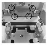
Align and attach with four hex screws. Make sure the cable is not pinched between the stacker and the assembly.
