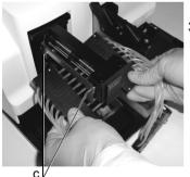
3) Hold the black left and the right dispensing cartridge below the rollers of the pump head, so that the tubings points downwards and the screws upwards. Fit the two holes on the inside of the left cartridge (<u>28</u>) with the two silver pins (c) located on the sliver lever. Position an equal number of tubes in front of and behind of the middle black roller wheel (<u>25</u>).
