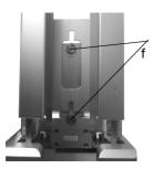
Connect the stacker chimneys by lowering them over the pins (f) on the chimney support brackets.
