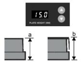
Enter the plate height (in mm) with the arrow keys on the front panel of the stacker.
