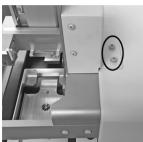
Align and attach top of assembly to top of stacker housing using two Philip head screws.
