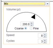
Selects the mixing volume by adjusting the dial or enter the volume directly.
