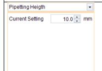
This will set a minimal Pipetting Height that limits vertical movement to that height. The Pipetting Height must be be activated by pressing the RUN button when this step is reached in the pipetting program.
