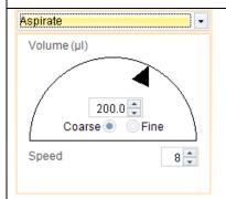
Use the dial to change the volume. To increase the volume in smaller increments, select "fine". Alternatively, you can enter the volume directly.
