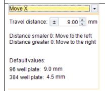
The plate or pipetting unit travels the set distance in X-direction relative to the current position.
