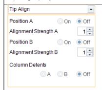
Activates tip align for the selected position. Tip align is an active positioning help to guide the pipette tips into the microplate wells.
