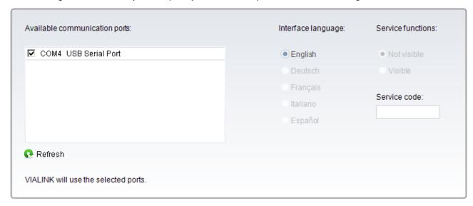
VIALINK will check the selected COM ports if a Programming Stand or instrument (MINI 96, VIAFLO 96, VIAFLO 384, ASSIST or ASSIST PLUS) is connected.
