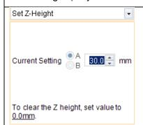
This will set a minimal Z-Height that limits vertical movement to that height. The Z-Height is activated when this step is reached in the pipetting program.
