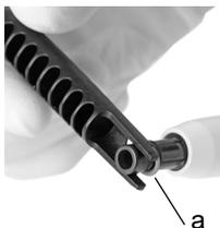
For 200 µl or 1000 µl pipettes, slide the multipurpose tool sideways onto the tip fitting until the O-ring (a) builds a loop. Remove the O-ring with plastic tweezers.
