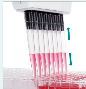
Pipet/Mix Transfer of a defined volume followed by a defined number of automatic mixing cycles
