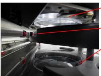
If the ground clearance is too low, the gripper cannot grip the base without lid.
