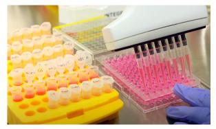
After saving the tip spacing, select 'Pipet' mode in the main menu. Set your required sample transfer volume
