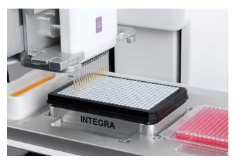
**Figure 4:** Example of the ASSIST PLUS pipetting robot transferring a master mix into a 384 well PCR plate.
