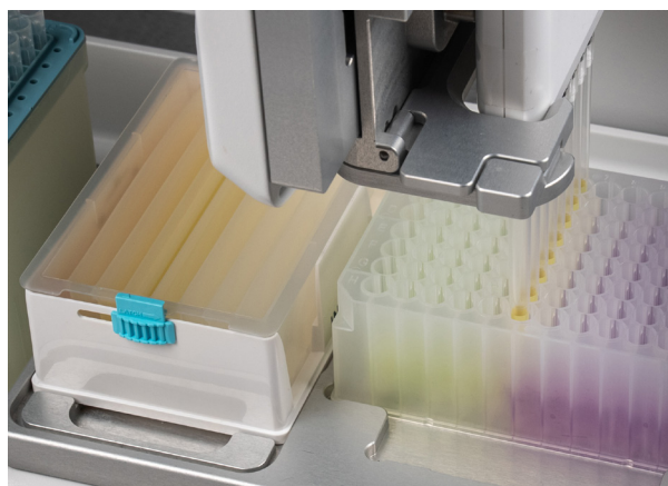
Figure 5: The VIAFLO on the ASSIST PLUS transferring a) ZymoPURE P3 to the DWP and b) the lysate to the ZymoPURE filter plate.
