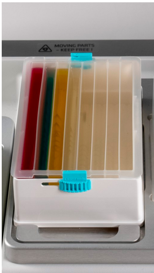
Figure 4: a) The 8 row divided reagent reservoir with base and reagents in portrait orientation on position A, and the VIAFLO transferring b) ZymoPURE P1 and c) ZymoPURE P2 to the DWP on the ASSIST PLUS.
