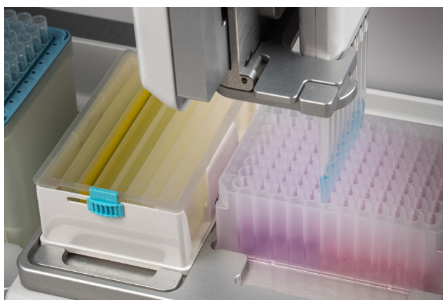
Figure 4: a) The 8 row divided reagent reservoir with base and reagents in portrait orientation on position A, and the VIAFLO transferring b) ZymoPURE P1 and c) ZymoPURE P2 to the DWP on the ASSIST PLUS.
