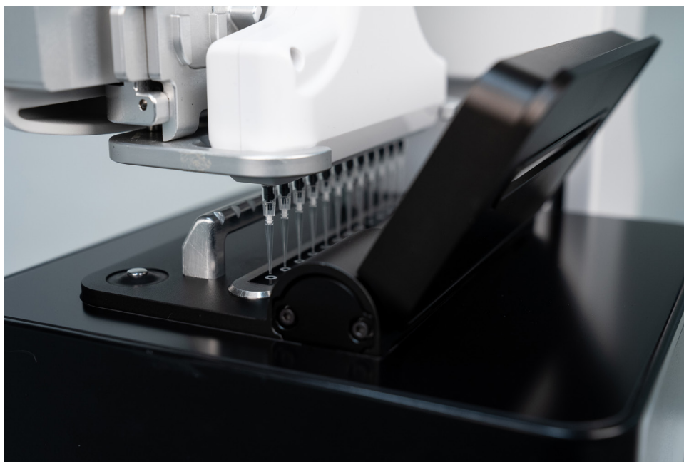
Figure 3: Automated sample loading onto the NanoPhotometer N120 with the ASSIST PLUS pipetting robot.
