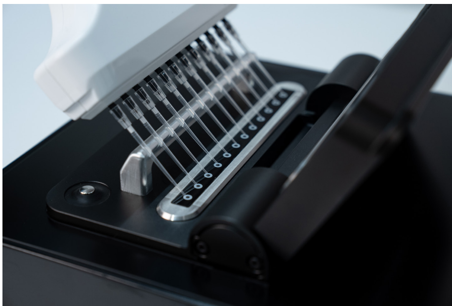
Figure 2: Manual sample loading onto the NanoPhotometer N120 with the help of the positioning guide.
