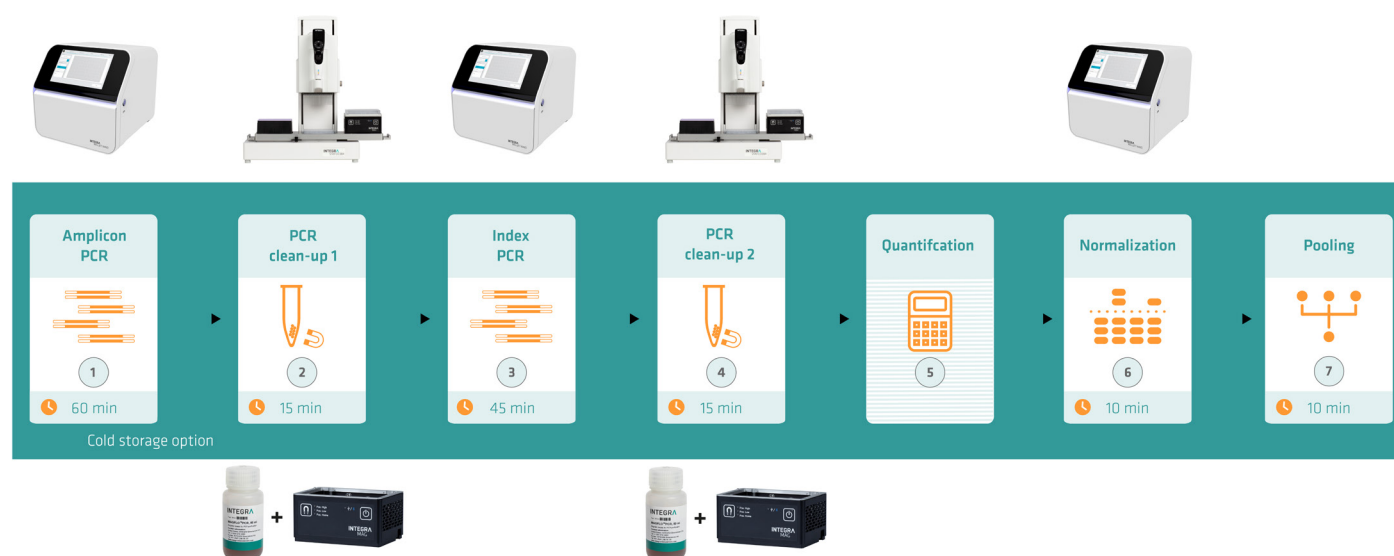
Figure 1: Overview of the 16S metagenome sequencing library preparation workflow (center) showing the use of the I.DOT LT and VIAFLO 384 (top), and the MAG module and MAGFLO™ NGS magnetic beads (bottom).
