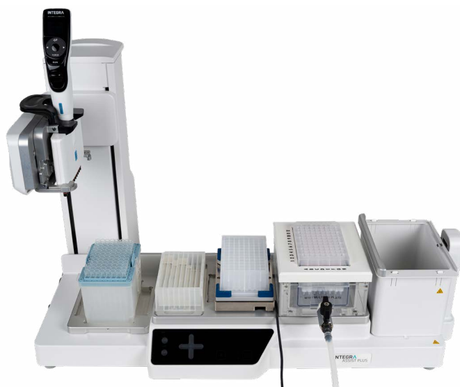
Figure 1: General set-up for the plasmid DNA purification program. Position A: 8 row reagent reservoir. Position B: 96 square-well block placed on the Teleshake microplate shaker. Position C: NucleoVac 96 Vacuum Manifold.
