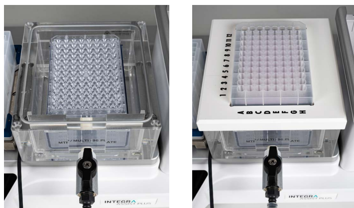
Figure 4: Vacuum manifold set-up for steps 5 and 6. The MN Wash Plate is inserted on the spacers inside the manifold base (left). The NucleoSpin Plasmid Binding Plate (white rings) with the cleared lysates is placed on top of the manifold (right).
