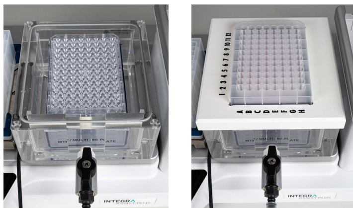
Figure 6: Vacuum manifold set-up for the elution step. The U-bottom elution plate is inserted on the spacers inside the manifold base (left). The NucleoSpin Plasmid Binding Plate (white rings) with the cleared lysates is placed on top of the manifold (right).
