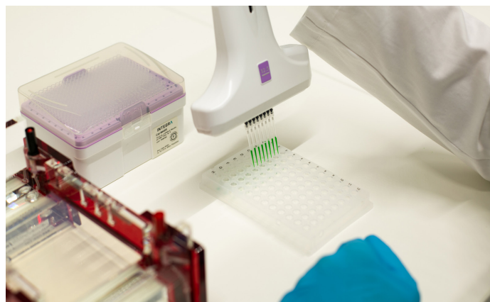
Figure 1: Sample transfer from a 96 well plate to an agarose gel. A) Sample aspiration from a 96 well plate using the VOYAGER 8 channel 12.5 µl electronic pipette with 9 mm tip spacing. B) Tip spacing is changed to 4.5 mm with the push of one button.
