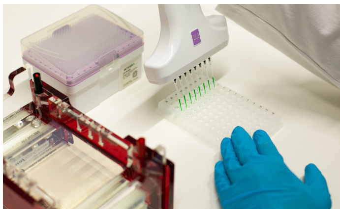
Figure 1: Sample transfer from a 96 well plate to an agarose gel. A) Sample aspiration from a 96 well plate using the VOYAGER 8 channel 12.5 µl electronic pipette with 9 mm tip spacing. B) Tip spacing is changed to 4.5 mm with the push of one button.
