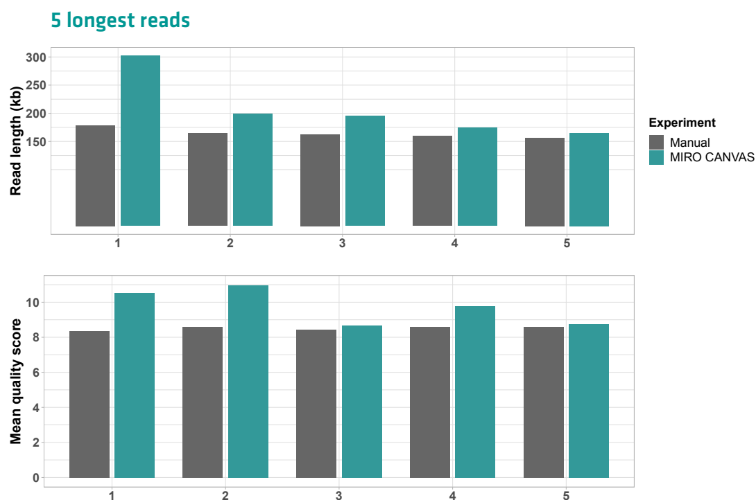
Figure 3: Read length and mean call base quality score for the five longest reads sequenced.
