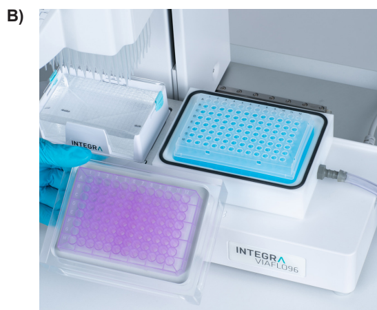
Figure 4: Elution into a) provided collection microtubes or b) a 96 well microplate.
