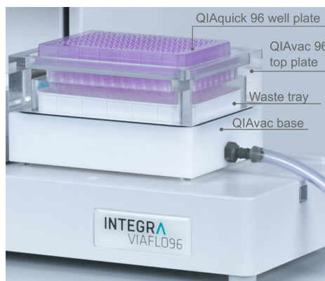
Figure 1: Initial set-up of the vacuum manifold.
