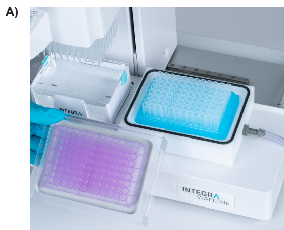
Figure 4: Elution into a) provided collection microtubes or b) a 96 well microplate.
