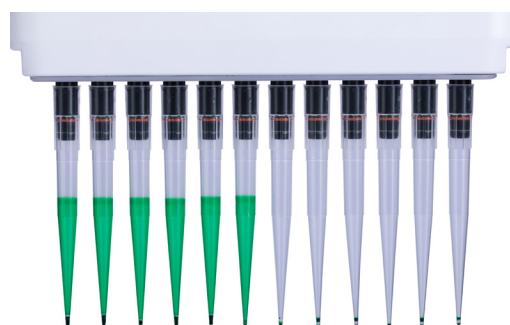
Figure 2: Pipetting a concentrated green dye with a 300 µl 12 channel VIAFLO electronic pipette featured with six standard GripTips (left) and six Low Retention GripTips (right).
