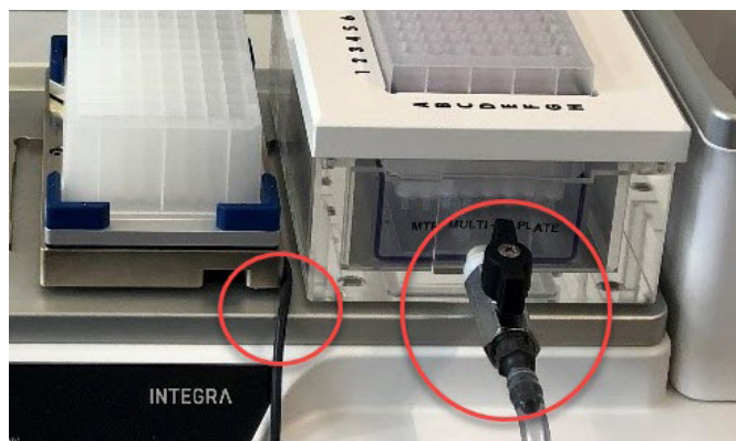
Figure 1: Positioning of the Teleshake cable and the outlet of the vacuum manifold.
