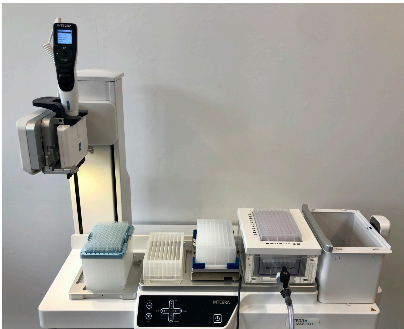
Figure 1: General set-up for the plasmid DNA purification program. Position A: 8 row reagent reservoir. Position B: Culture Plate (96 Square-well Block) placed on the Teleshake microplate shaker. Position C: NucleoVac 96 Vacuum Manifold.
