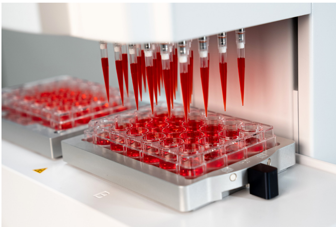
Figure 9: Sample transfer between 24 well plates with the VIAFLO 96 handheld electronic pipette equipped with a 24 channel pipetting head.
