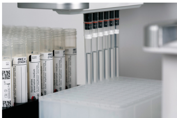
Figure 3: Sample transfer from a) swab tubes to b) 96 deep well plate with VOYAGER pipette.
