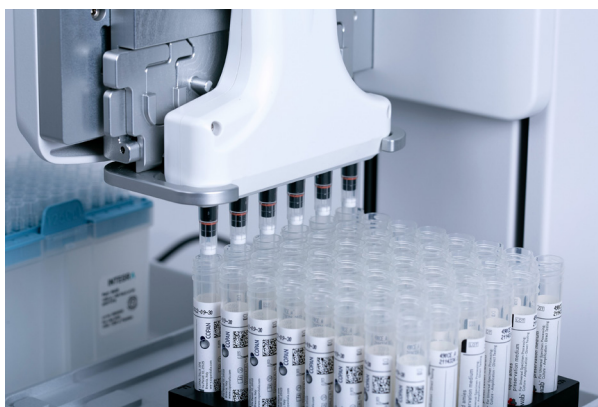
Figure 3: Sample transfer from a) swab tubes to b) 96 deep well plate with VOYAGER pipette.
