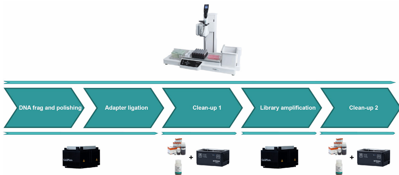
Figure 1: Schematic representation of the sparQ DNA Frag & Library Prep Kit workflow showing the use of the ASSIST PLUS pipetting robot (top), the individual steps of the workflow (center) and the use of the COLDPLATE, MAG module and sparQ PureMag Beads (Quanta bio ) or MAGFLO NGS beads (INTEGRA Biosciences) (bottom).
