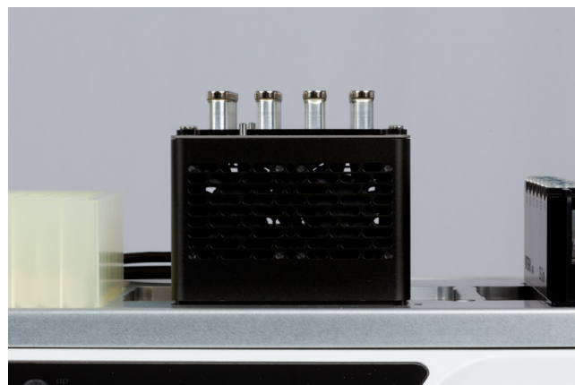
Figure 4: The HEATMAG module on the ASSIST PLUS without a tube adapter, showing (a) the disengaged magnet array (home position, 0 mm) and (b) the engaged magnet array (high position, 29 mm).
