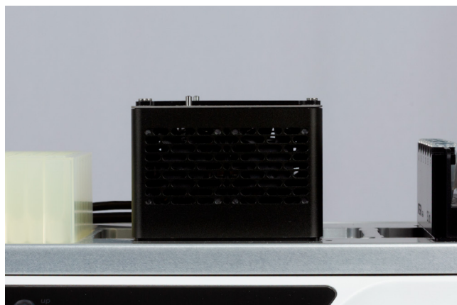
Figure 4: The HEATMAG module on the ASSIST PLUS without a tube adapter, showing (a) the disengaged magnet array (home position, 0 mm) and (b) the engaged magnet array (high position, 29 mm).
