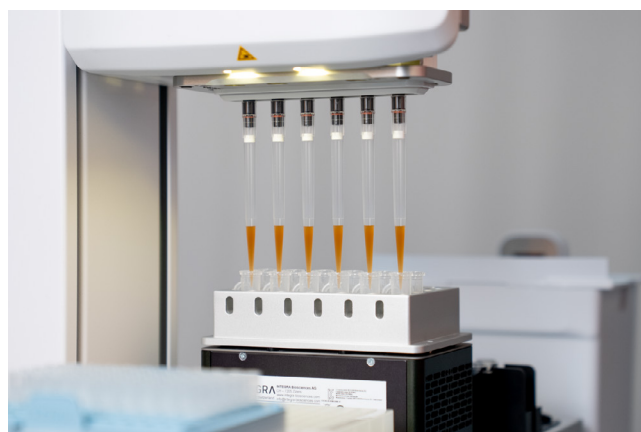
Figure 3: The VOYAGER on the ASSIST PLUS transfers the Blood DNA Particle Solution from (a) the DWP with reagents to (b) the 1.5 ml microcentrifuge tubes containing lysates on the HEATMAG module equipped with a 24 position tube adapter.
